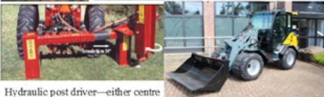
Hydraulic post driver—either centre mounted or offset behind tractor. Also available mounted on Weidemann loader
